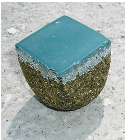
Fig. 8 G9 glass coated Foamglas ® after 6 h of erosion test (modification of Uni En Iso 10545-7, measured by Turbula T60). Original sample size: 30 \times 30 \times 30 \text{ mm}^3
